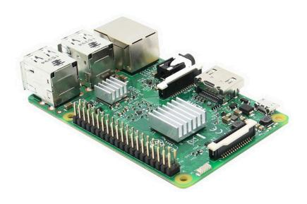
While the small heatsinks help they are insufficient for creating a high reliability embedded controller. With the height restriction removed we are free to add heatsinks with far greater heights and therefore far greater surface areas to distribute heat.
