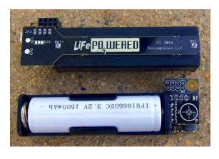
provides these capabilities. The battery used is a standard 18650 form factor cell which snaps into a standard cell holder for easy replacement in 15 years. Chemical systems like batteries don't last forever.
